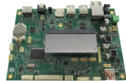
Passive cooling for use with Box-Set
