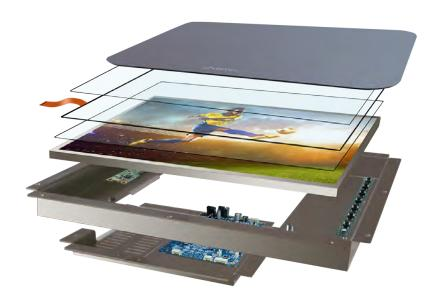
Branded as our VacuBond service, the dry bonding method is used at Display Technology Ltd.
