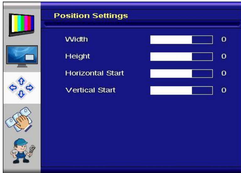
Figure 6.3.a: "Position Settings" menu for video mode of HDMI, S-Video, composite and component inputs.
