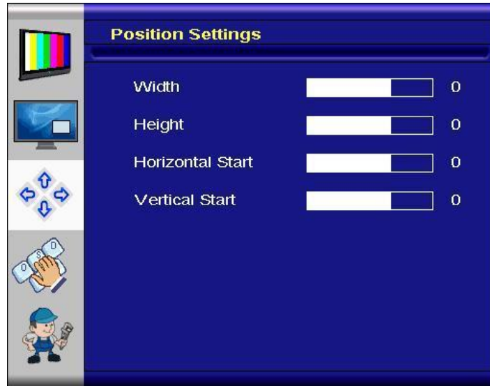
Figure 6.3.a: “Position Settings” menu for video mode of HDMI, S-Video, composite and component inputs.
