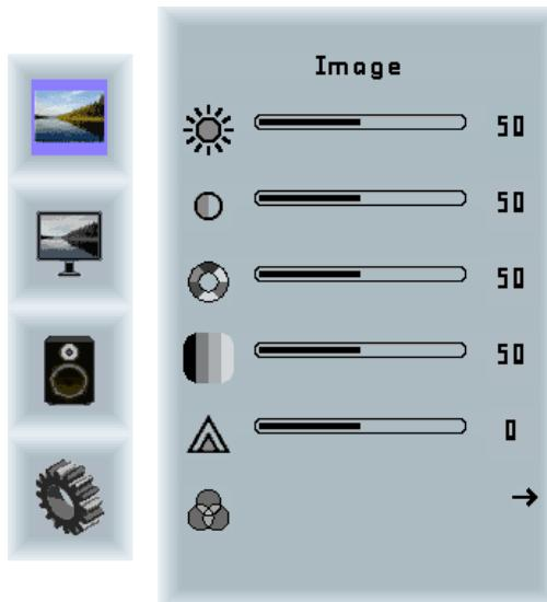
**Brightness:** Brightness of the image can be controlled using this function, with left and right buttons after the brightness slider is selected. This function modifies RGB data to change the brightness.
