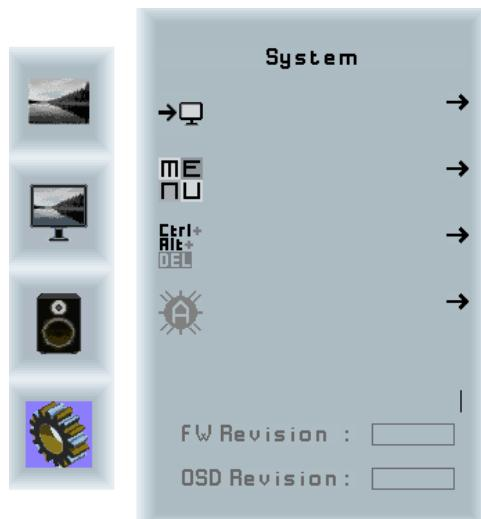
If there is no Auto Brightness sensor is available, Auto Brightness icon is either not shown or non-selectable according to the firmware version.
