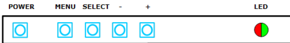
Figure 2: External 4 Button OSD Keypad ZU-02-315
