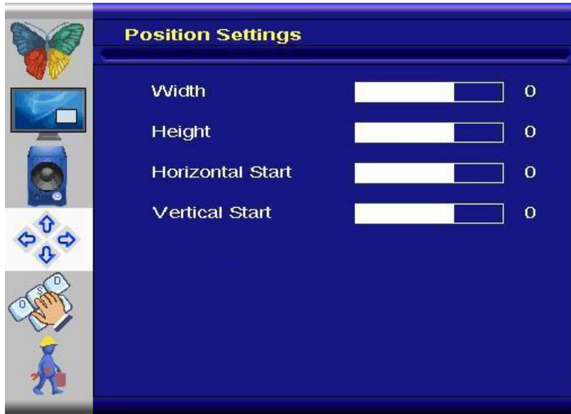
Figure 7.4.a "Position Settings" menu for video mode of HDMI, s-video, composite and component inputs.
