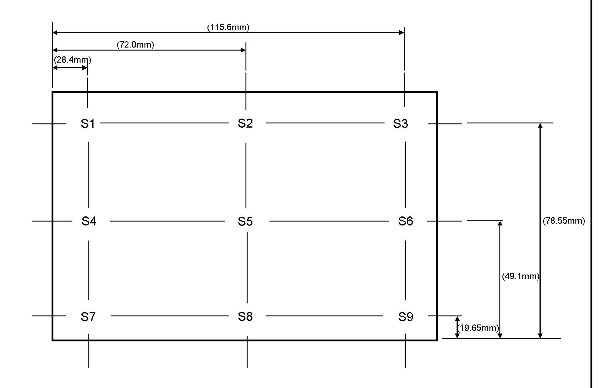
$$\begin{array}{c} \text{Minimum Value of S1-S9} \\ \text{Standard Value of Brightness Uniformity [\%]} = & \\ \hline & \\ \text{Maximum Value of S1-S9} \\ \end{array}$$
