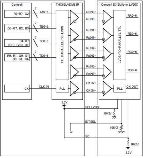
$\mbox{\ensuremath{\$}SELLVDS}$  signal line has 10 k  $\Omega$   $\,$  pulldown resister.
