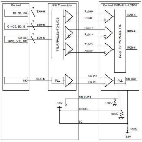
$\mbox{\ensuremath{\$}SELLVDS}$  signal line has 10 k  $\Omega$   $\,$  pulldown resister.
