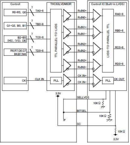
$\ensuremath{\texttt{SELLVDS}}$  signal line has 10 k  $\Omega$   $\ensuremath{\,\text{pulldown}}$  resister.
