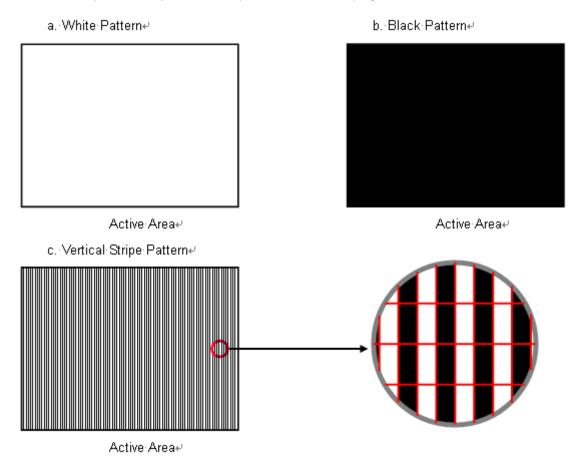
Note (4) The power consumption is specified at the pattern with the maximum current.
