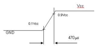
Note (3) The specified power supply current is under the conditions at Vcc = 3.3 V, Ta =  $25 \pm 2$  °C, Fr = 60Hz, whereas a power dissipation check pattern below is displayed.
